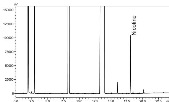
Figure 3: Example chromatogram of the e-liquid sample. The other major peaks are likely to be methanol (solvent), propylene glycol and glycerin
