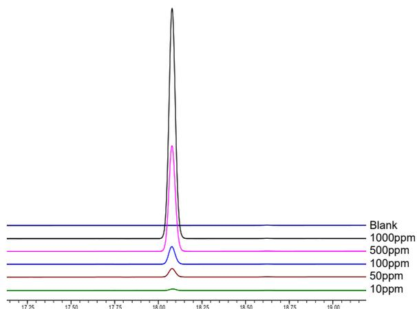
Figure 2: Chromatograms of nicotine standards. The blank was run after the 1000ppm triplicate runs
