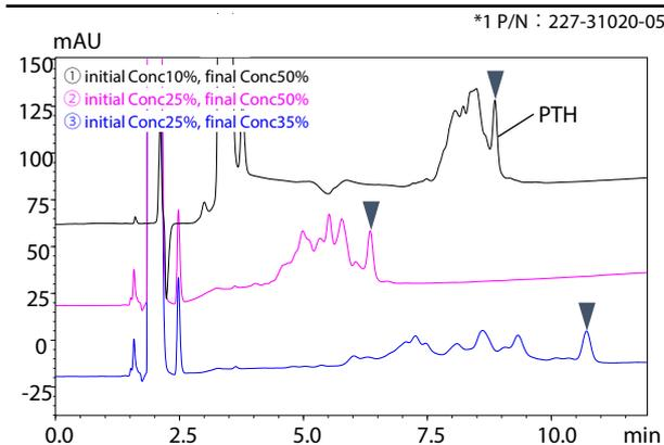
Fig. 2 Result of optimization for separation conditions
