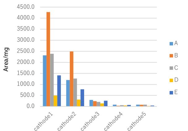
Fig.8 Comparison of residual solvent levels from five different NCM cathodes with different drying processes (n=3 average)
