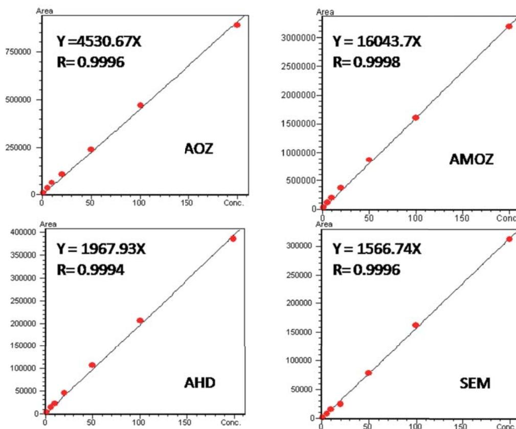
Fig. 5 Calibration curve of 4 derivatives of nitrofurantoin metabolites
