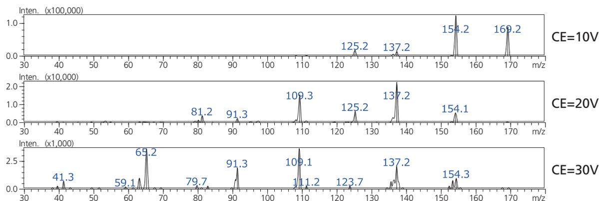
Figure 5 Product ion scan spectra of E6 standard
