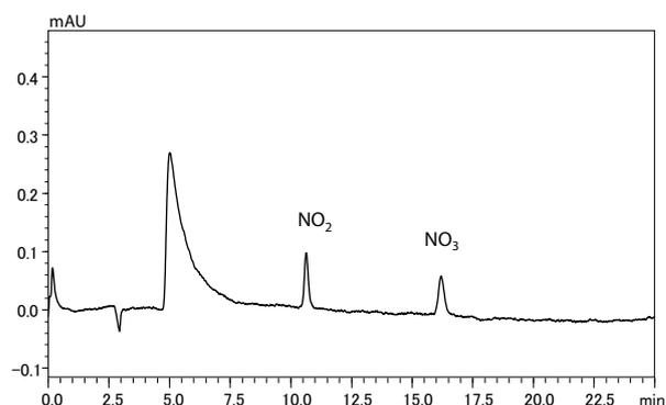
Fig.2 Chromatogram of Standard Nitrate and Nitrite Ions
