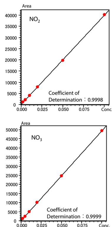
Fig.3 Calibration Curves for Nitrate and Nitrite Ions
