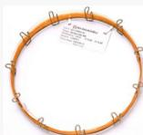
Column lifetime can vary depending on the type of column, usage condition and sample quality. Chromatographic issues (e.g. change in retention time, decrease resolution, decreased sensitivity etc.) are indication for replacing of column.
