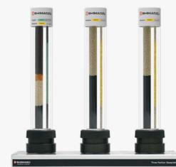
Impurities in gases, such as hydrocarbons, moisture and oxygen, can contaminate the gas line and instrument, cause column degradation and affect the accuracy of your analysis results, which may lead to instrument downtime. Even with high-purity gases, contaminants may come from pressure regulators or other parts of the gas line. Therefore, gas filter is essential to ensure high quality gas is used for GC analysis.
