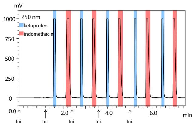
Fig 5. Preparative SFC chromatogram “stacked Injection mode”
