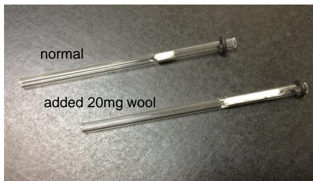
Figure 2: Positioning of additional silica wool in glass insert for aqueous analysis. The additional wool was packed more loosely than the originally supplied portion, as overly compact wool might create unnecessarily high pressure within the injector port during use.
