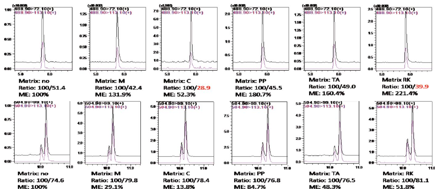
Fig. 3: Comparison of peak intensity ratios and matrix effect values for vardendafil (top) and thiodimethylsildenafil (bottom) in different sample matrices.
