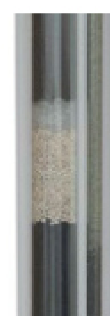
If absorbent is saturated, the indicator changes color
